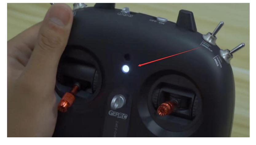
• The middle indicator light keeps flashing, which means that the remote control is ready. Then you can put the remote control aside and let it flashing. Next, we take out the Drone and go to the next step
