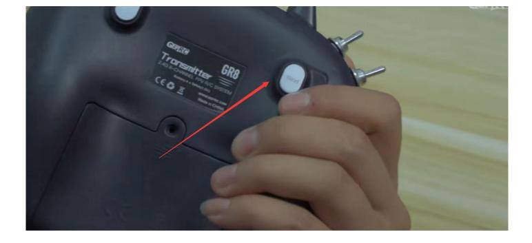
Press and hold the bind button on the back with your fingers, and then turn on the remote control
