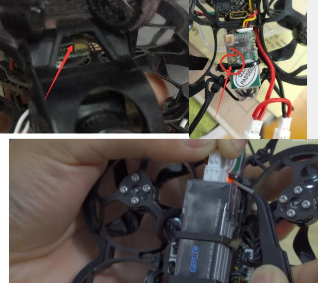
Press and hold the frequency key of the receiver with tweezers, later connect the two batteries of the Drone. The drone and remote controller can be bind automatically. After binding, the indicator light of the remote control is always on
